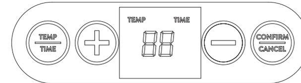
TEMP button = Press the "Temp" button to select one of the temperatures from 25°C to 50°C, press "+/-" button to adjust the temperature with 1 degree increments.
